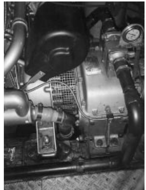
CENTAMAX-B for main propulsion between Diesel engine on soft mounts and marine gear on rigid mounts.
